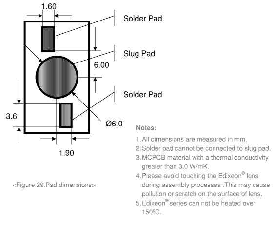
The choice of solder and the application method will dictate the specific amount of solder. For most consistent results, an automated dispensing system or a solder stencil printer is recommended.
