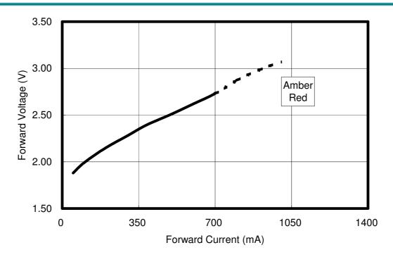
Figure 17 Forward current & forward voltage for 3W Edixeon  $^{\rm @}$  series at T\_J=25 $^\circ\!{\rm C}\,{>}$
