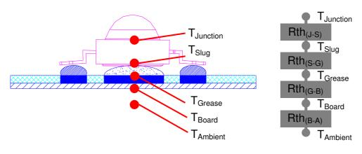
$Rth_{(J-A)} = Rth_{(J-S)} + Rth_{(S-G)} + Rth_{(G-B)} + Rth_{(B-A)}$
