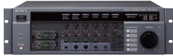
SRP-X500P with two URX-M2 tuner modules installed
